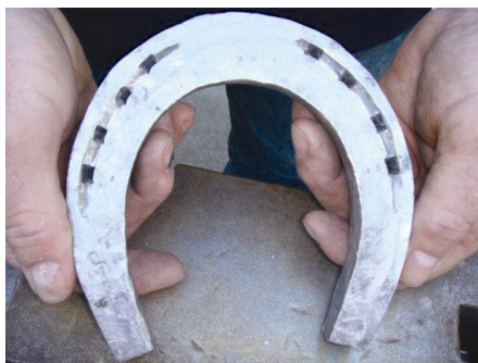
Eggbar wedge blank welded and wear bar
